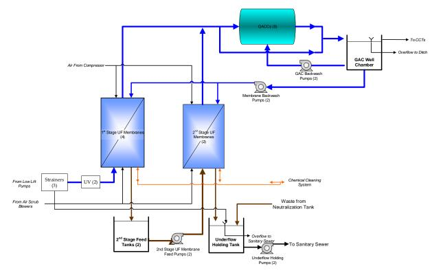
A schematic of new treatment system is provided below.
